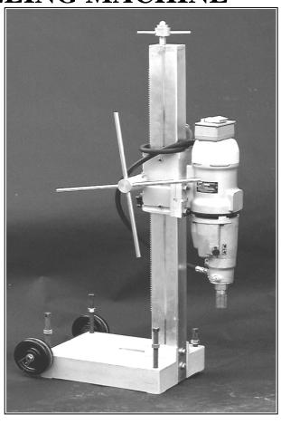
**MOTOR:** Either a Core Bore or Milwaukee 20 Amp. 2 speed motor is available. Both feature ball and roller bearings and hardened triple reduction gearing for long life. All motors contain a built in water swivel to direct water through the bit. CB motors feature a clutch to prevent overload. Milwaukee motors are available with a clutch or shear pin for overload protection.
