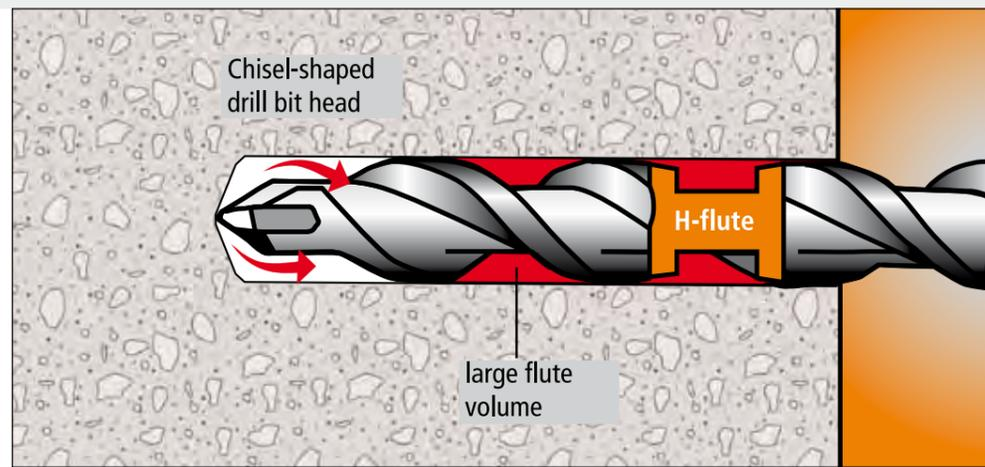
**PGM conformity** stands for precisely fitting anchor holes and precise concentricity.
